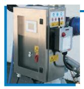
A-60 industrial dust suppression fog cannon: control panel with remote control detail.
