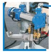
Water distribution by solenoid valves and water filter installed on the A-60 industrial dust suppression fog cannon: 60
